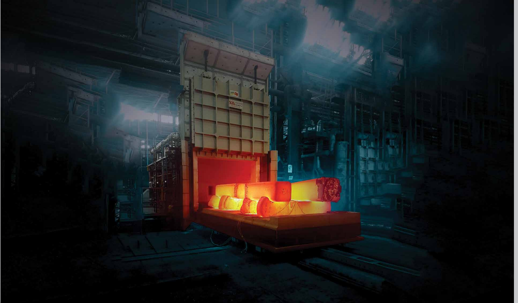
ARABA VEYA SABİT TABANLI ISIL İŞLEM FIRINLARI BOGIE HEARTH OR FIXED BOTTOM TYPE HEAT TREATMENT FURNACES
